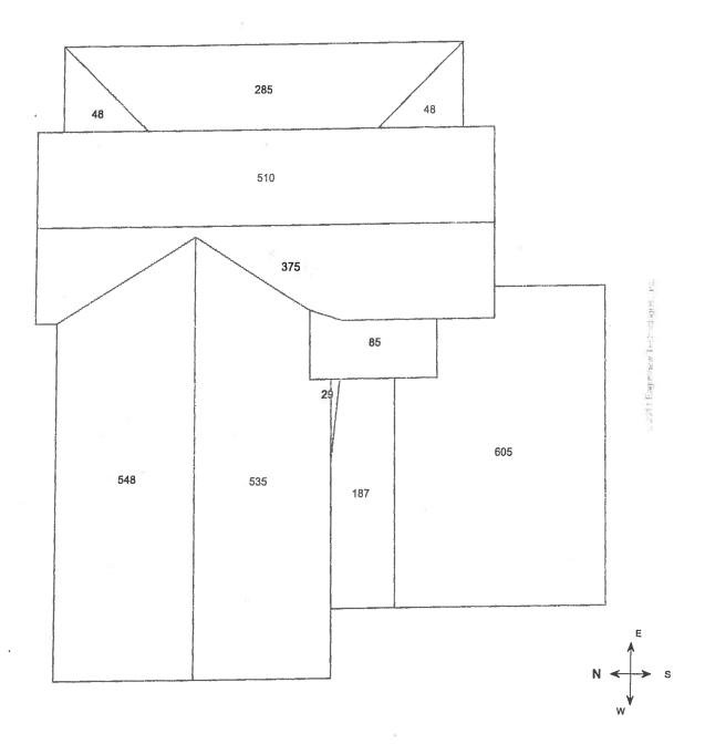
Note: This diagram shows the square feet of each roof facet (rounded to the nearest foot). The total area in square feet, at the top of this page, is based on the non-rounded values of each roof facet (rounded to the nearest square foot after being totaled).
