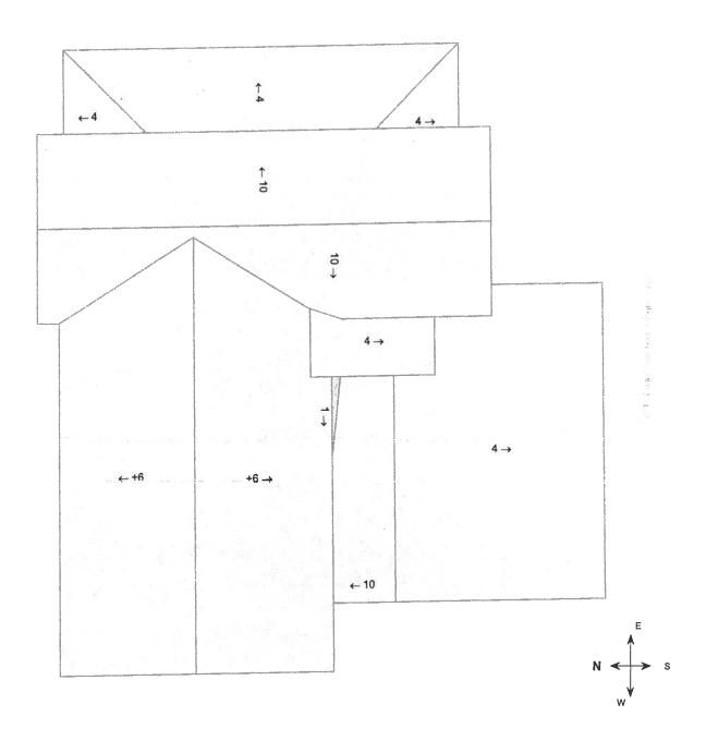
Note: This diagram contains labeled pitches for facet areas larger than 20 square feet. In some cases, pitch labels have been removed for readability. Blue shading indicates a pitch of 3/12 and greater. Gray shading indicates flat, 1/12 or 2/12 pitches.
