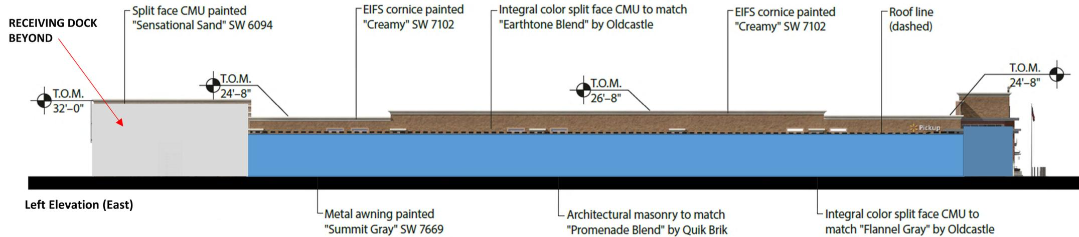
**TOTAL AREA OF SIDE FAÇADE UNDER ROOF = 5,694 SF      5,694 SF X .20 = 1,139 SF OF GLASS REQUIRED**
